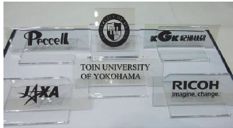
Ink-jet printed patterns of perovskite films
